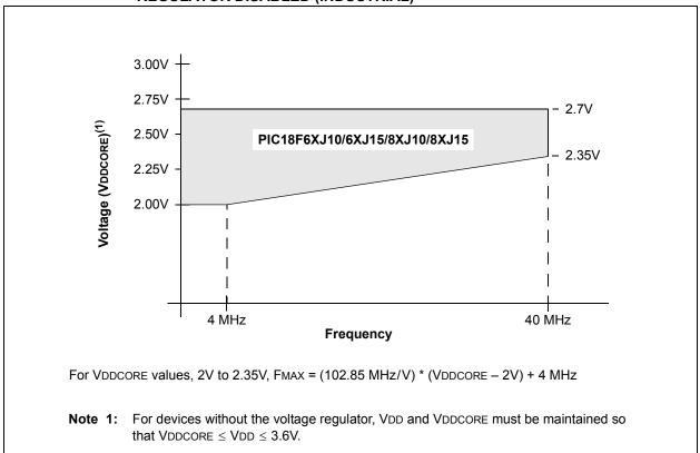
FIGURE 27-2: PIC18F87J10 FAMILY VOLTAGE-FREQUENCY GRAPH, REGULATOR ENABLED (INDUSTRIAL)
