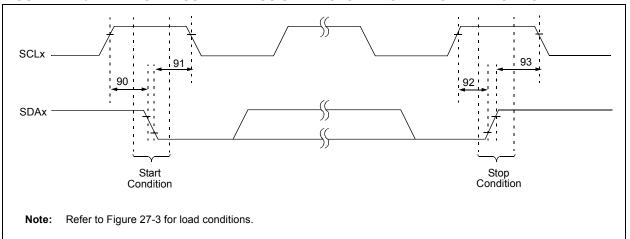
TABLE 27-22: MASTER SSP I<sup>2</sup>C™ BUS START/STOP BITS REQUIREMENTS
