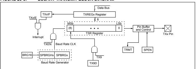
FIGURE 20-4: ASYNCHRONOUS TRANSMISSION
