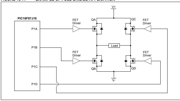
FIGURE 18-7: EXAMPLE OF FULL-BRIDGE APPLICATION
