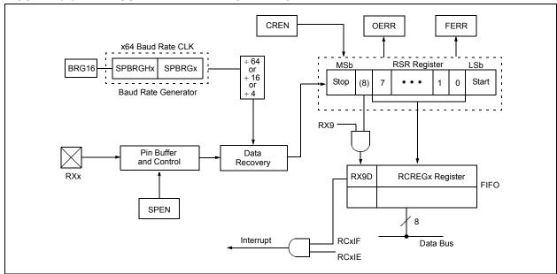
FIGURE 20-7: ASYNCHRONOUS RECEPTION
