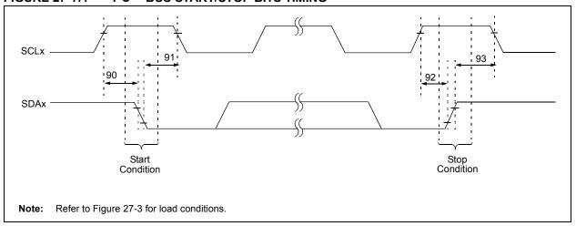
TABLE 27-20: I<sup>2</sup>C™ BUS START/STOP BITS REQUIREMENTS (SLAVE MODE)
