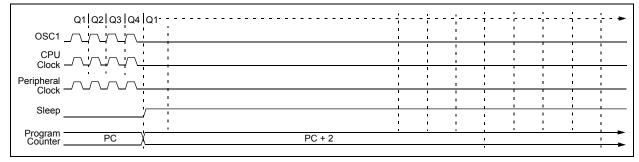
FIGURE 4-6: TRANSITION TIMING FOR WAKE FROM SLEEP (HSPLL)
