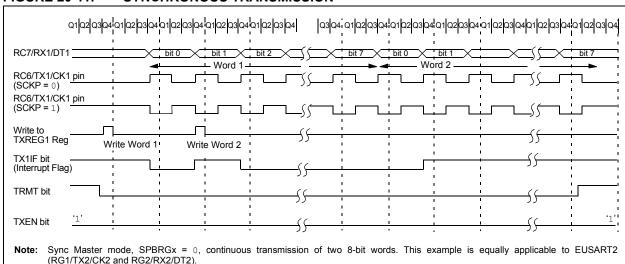
FIGURE 20-12: SYNCHRONOUS TRANSMISSION (THROUGH TXEN)
