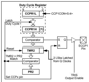
Note 1: The two LSbs of the Duty Cycle register are held by a 2-bit latch that is part of the module's hardware. It is physically separate from the CCPR registers.
