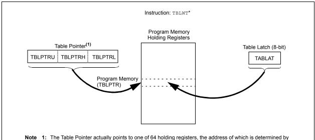
The Table Pointer actually points to one of 64 holding registers, the address of which is determined by TBLPTRL<5:0>. The process for physically writing data to the program memory array is discussed in Section 7.5 "Writing to Flash Program Memory".
