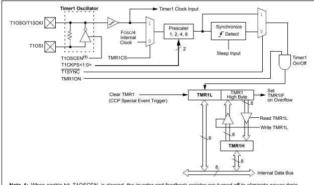
Note 1: When enable bit, T10SCEN, is cleared, the inverter and feedback resistor are turned off to eliminate power drain.
