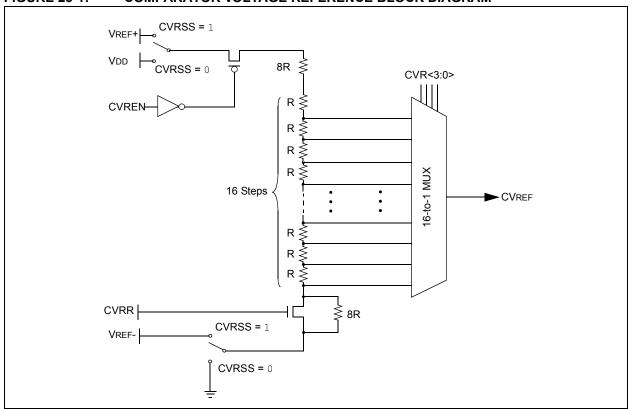
FIGURE 23-1: COMPARATOR VOLTAGE REFERENCE BLOCK DIAGRAM
