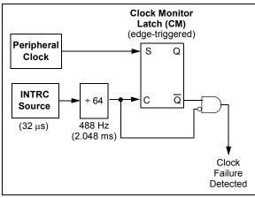
Clock failure is tested for on the falling edge of the sample clock. If a sample clock falling edge occurs while CM is still set, a clock failure has been detected (Figure 24-5). This causes the following:
