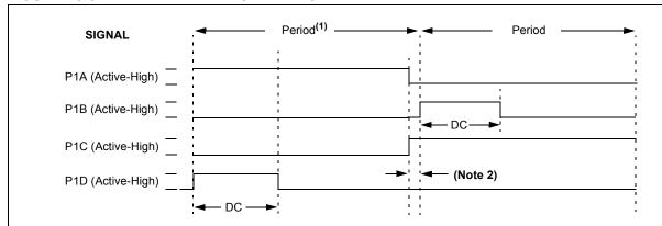
Note 1: The direction bit in the ECCP1 Control register (CCP1CON<7>) is written at any time during the PWM cycle. 2: When changing directions, the P1A and P1C signals switch before the end of the current PWM cycle at intervals of 4 Tosc, 16 Tosc or 64 Tosc, depending on the Timer2 prescaler value. The modulated P1B and P1D signals are inactive at this time.
