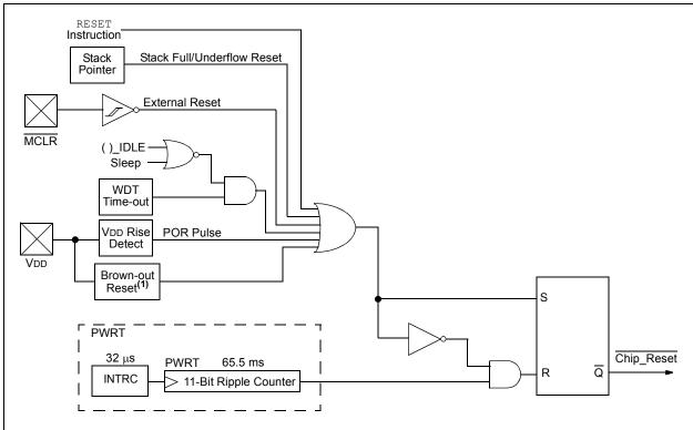
**Note 1:** The ENVREG pin must be tied high to enable Brown-out Reset. The Brown-out Reset is provided by the on-chip voltage regulator when there is insufficient source voltage to maintain regulation.
