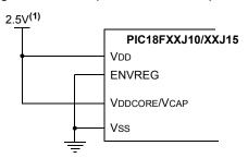
Note 1: These are typical operating voltages. Refer to Section 27.1 "DC Characteristics: Supply Voltage" for the full operating ranges of VDD and VDDCORE.
