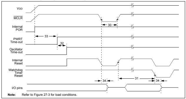
TABLE 27-12: RESET, WATCHDOG TIMER, OSCILLATOR START-UP TIMER, POWER-UP TIMER AND BROWN-OUT RESET REQUIREMENTS
